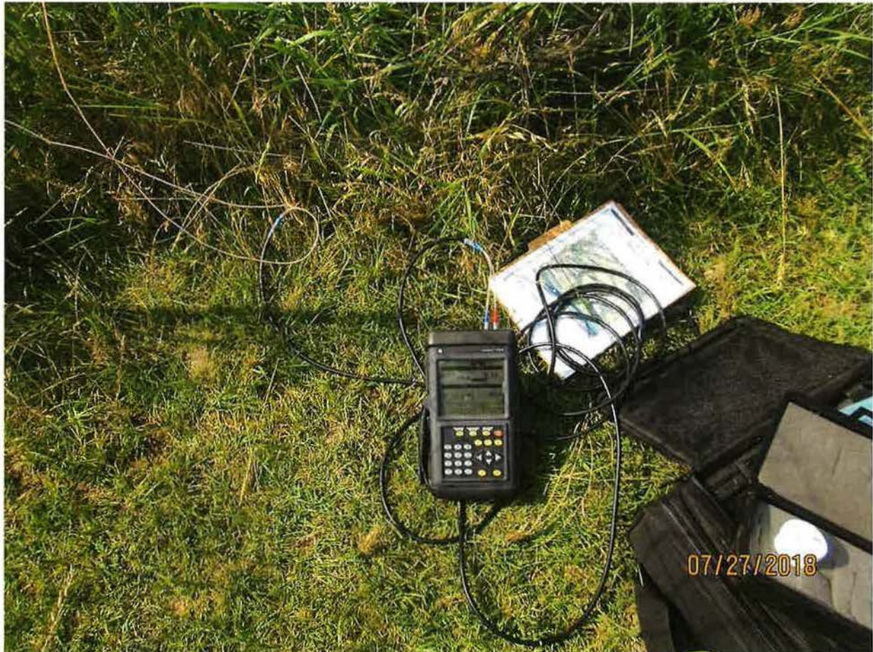
Flow measurement taken using GE Panametric Ultrasonic Flowmeter.
