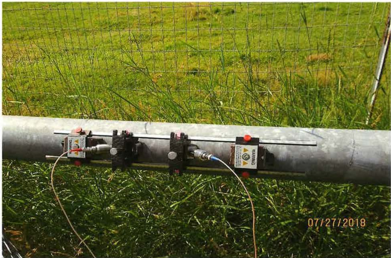
Flow measurement taken using GE Panametric Ultrasonic Flowmeter.
