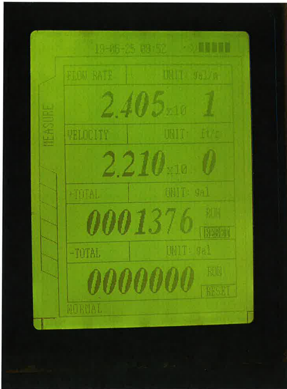
Figure 5: An example of an instantaneous flow rate on the meter readout screen.
