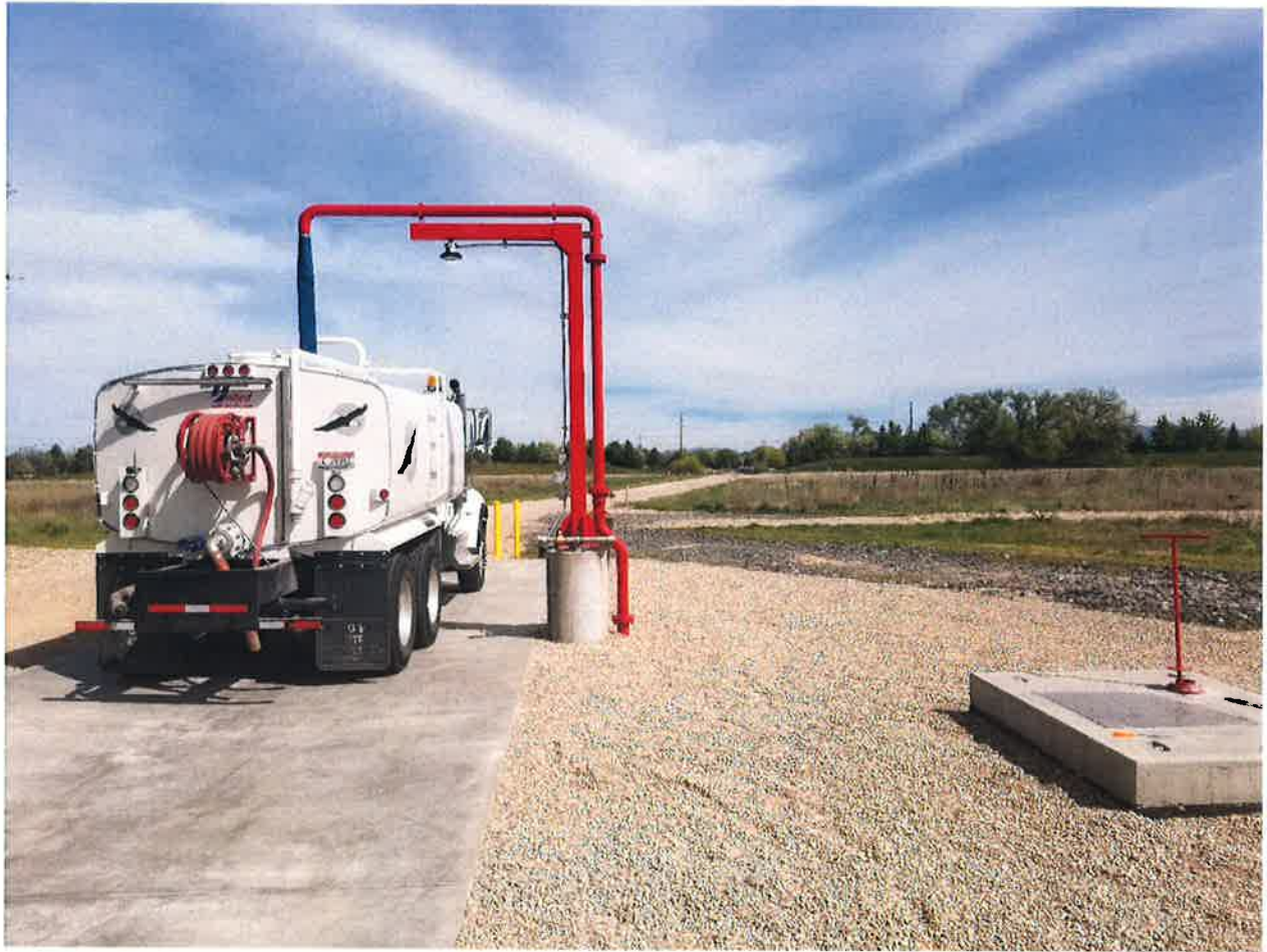
4,000 gallon water tanker truck used to haul water for sewer cleanouts.
