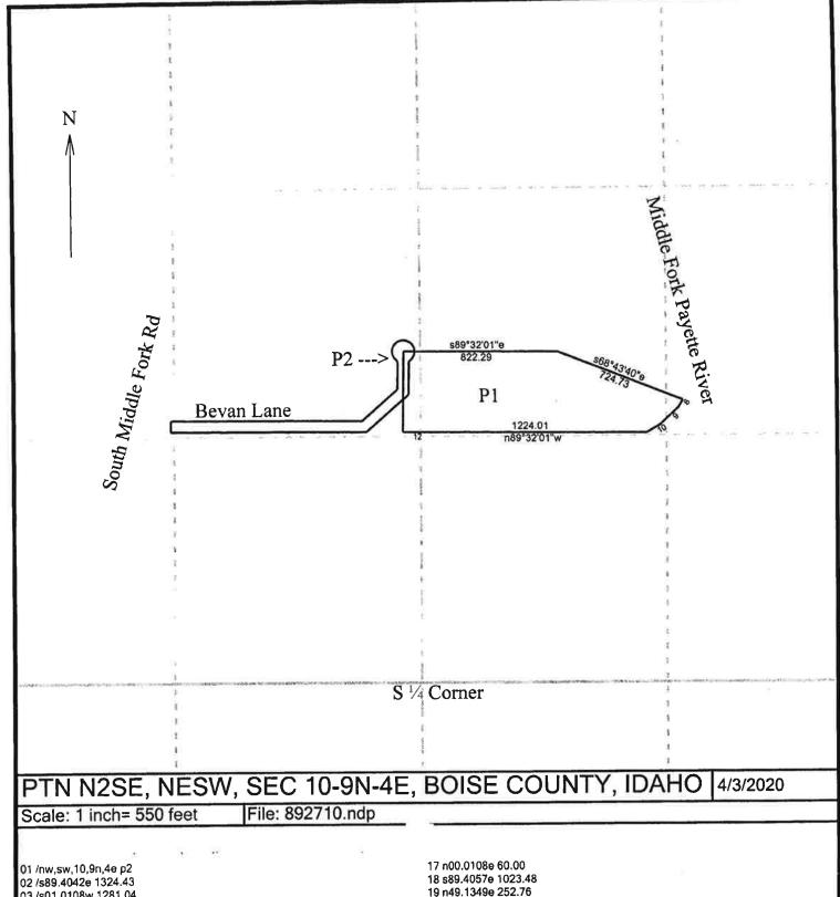
03 /s01.0108w 1281.04 04 /s89.4057e 1242.45 05 n00.5329e 430.23 06 s89.3201e 822.29 07 s68.4340e 724.73 08 s32.1450w 48.75 09 s47.1918w 129.39 10 s60.3051w 85.44 11 n89.3201w 1224.01 12 n89.4057w 84.84 13 @0 ESMT 14 /nw,sw,10,9n,4e 15 /s89.4042e 1324.43
