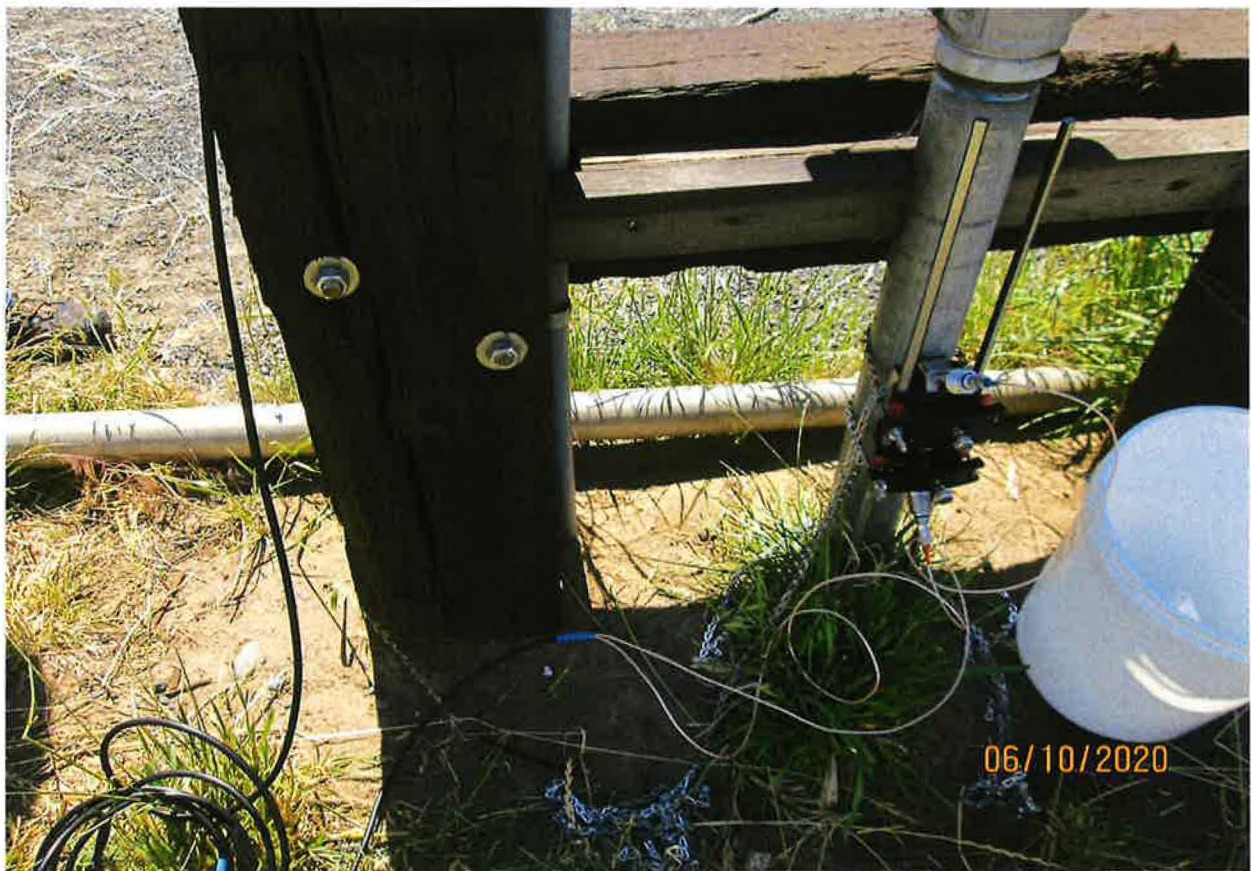
FLOW MEASUREMENTS FROM MAIN BEAM IRRIGATION PIPE FROM PUMP
