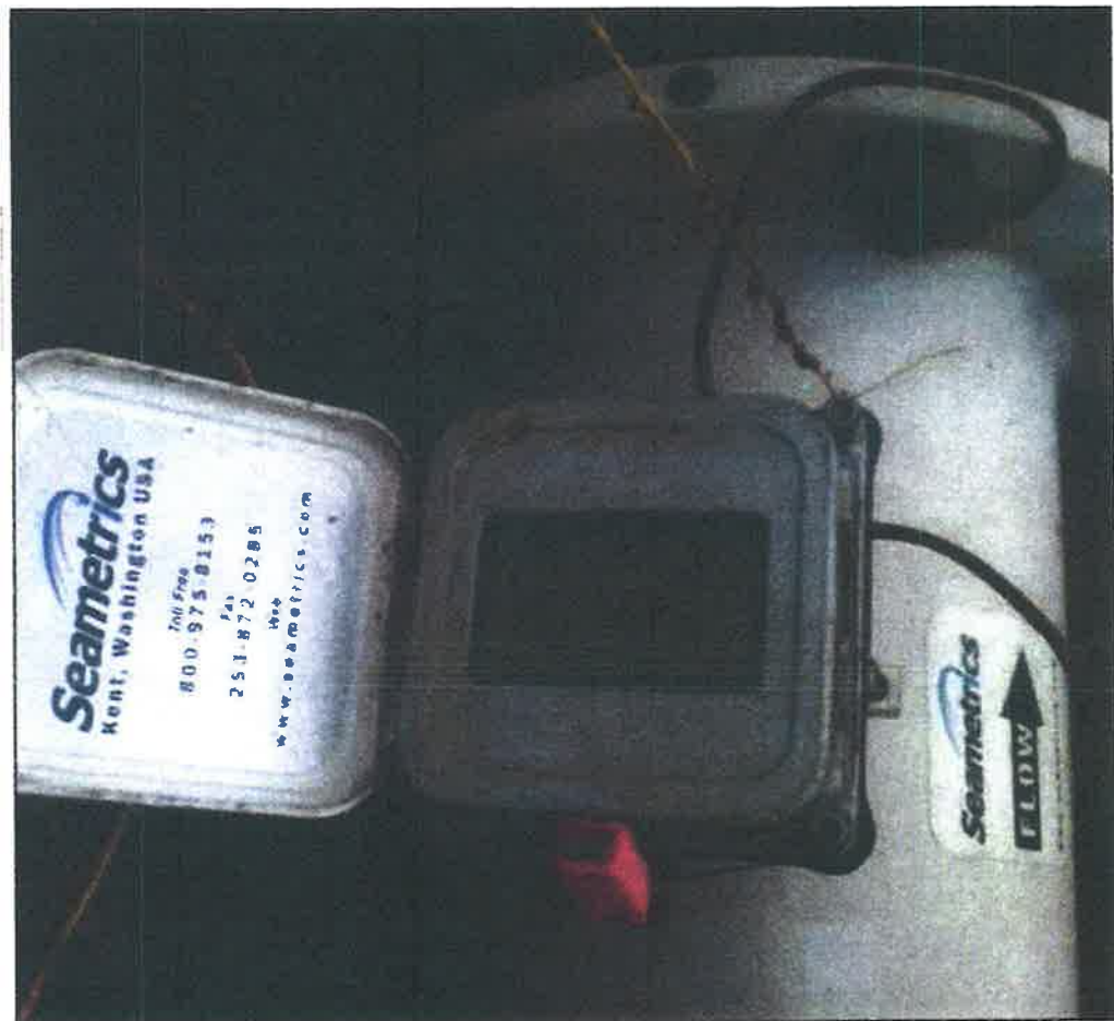
2-14-2014 CDN #4 Pivot/Reservoir flow-meter not suitable for the intended purpose; especially at lower flows.
