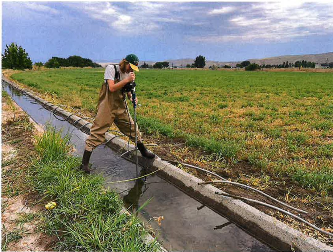
Fig. 9 – WR agent Tyler Smith conducting a flow measurement in open ditch.
