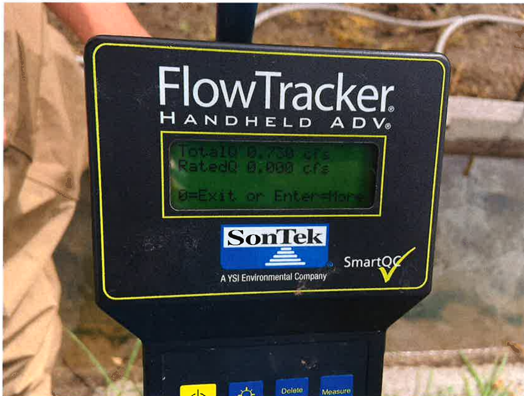
Fig. 10 – Results of FlowTracker measurements yielded a rate of 0.73 cfs.
