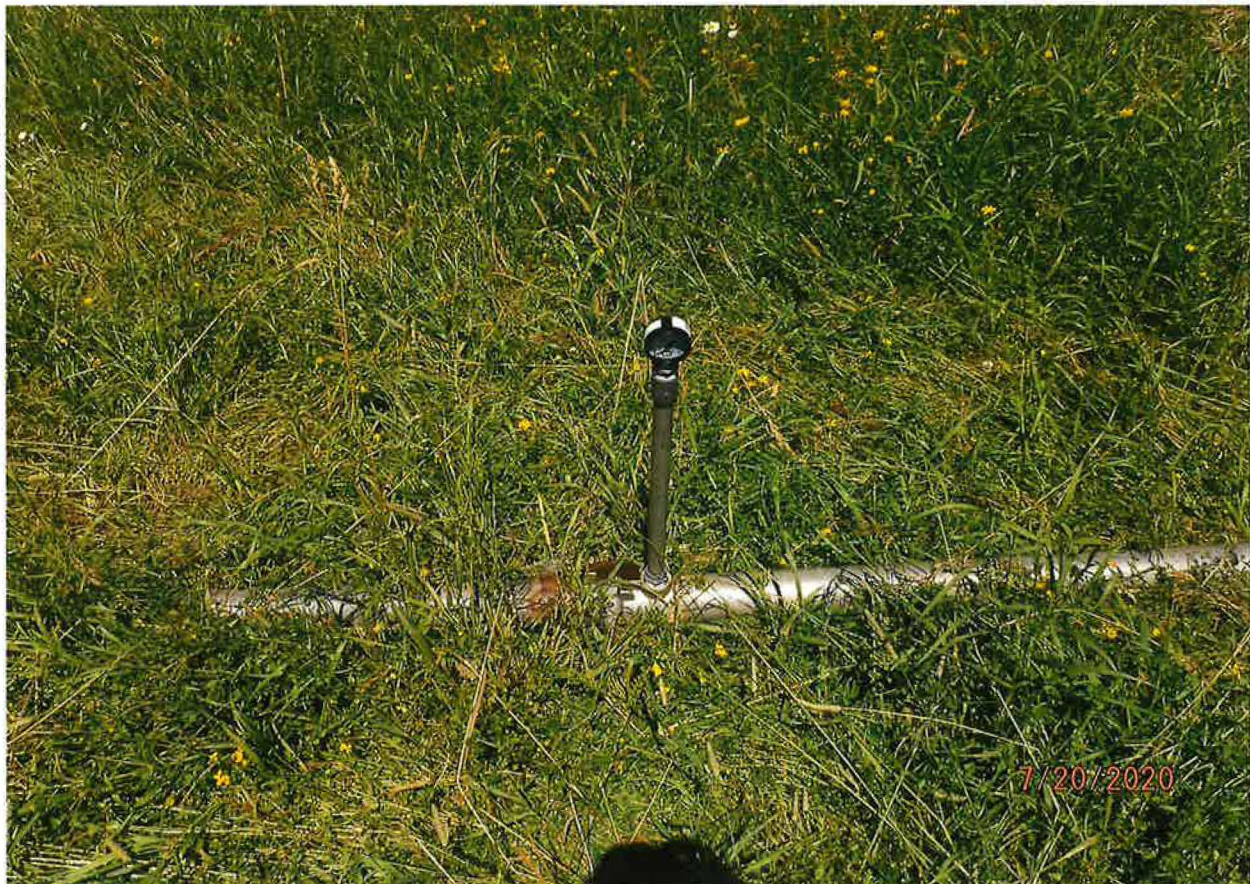
IRRIGATION PSI AT TIME OF OPERATION = AVG 25 PSI
