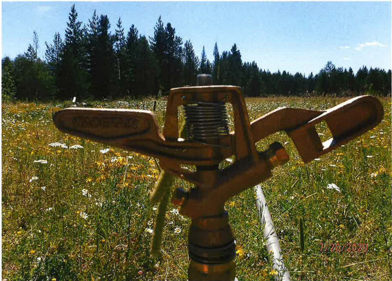
IRRIGATION SPRINKLERS – 10EA 7/32 ND AND 1EA 5/32 ND NOZZLES
