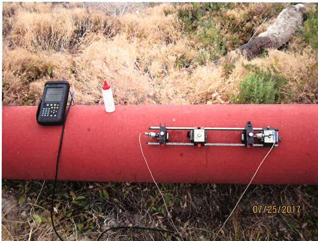
Figure 7. The transducers and Panametric measuring device attached to the 18 inch steel diversion pipe at the measuring site.
