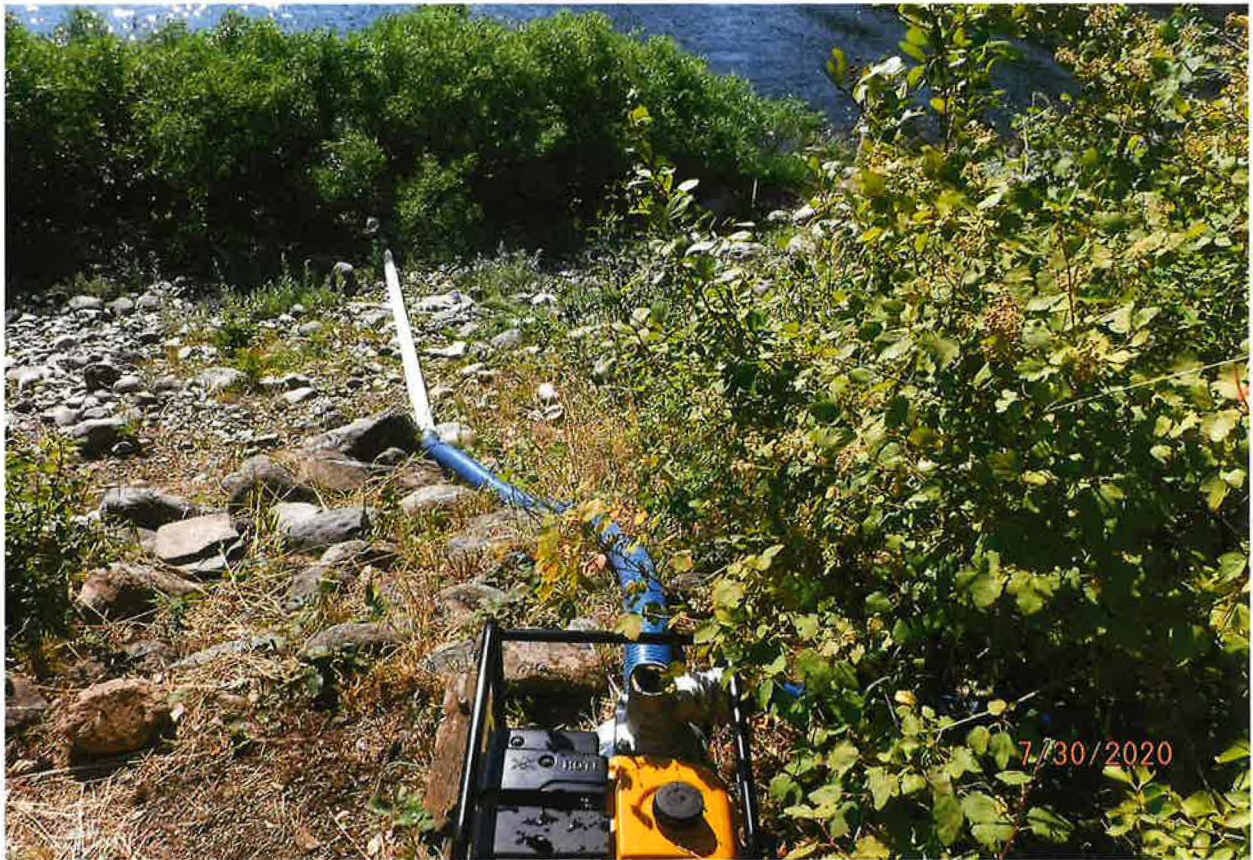
3 INCH PVC PIPE FROM POD UPHILL TO WATER TRANSFER PUMP
