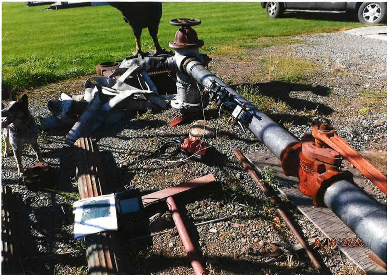
FLOWMETER MEASUREMENT FOR DIVERSION RATE
