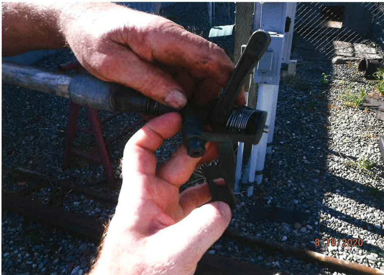
5/32 ND NOZZLE SPRINKLER – 32EA IN OPERATION AT ONE TIME
