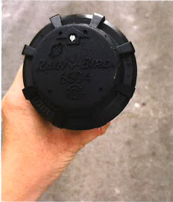
Rain Bird 6504 Rotors, typically irrigate using 24 heads per section, the POU consists of 6 sections.
