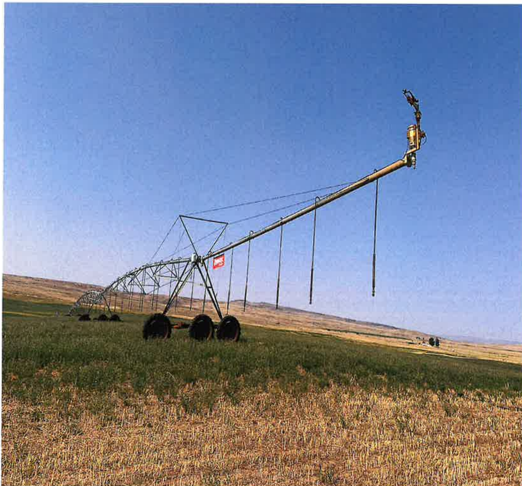
Fig. 4 – 7 TWR ZIMMATIC 9500 FC pivot. The NE and SE sections of this permit's place of use are irrigated with the pivot end gun.
