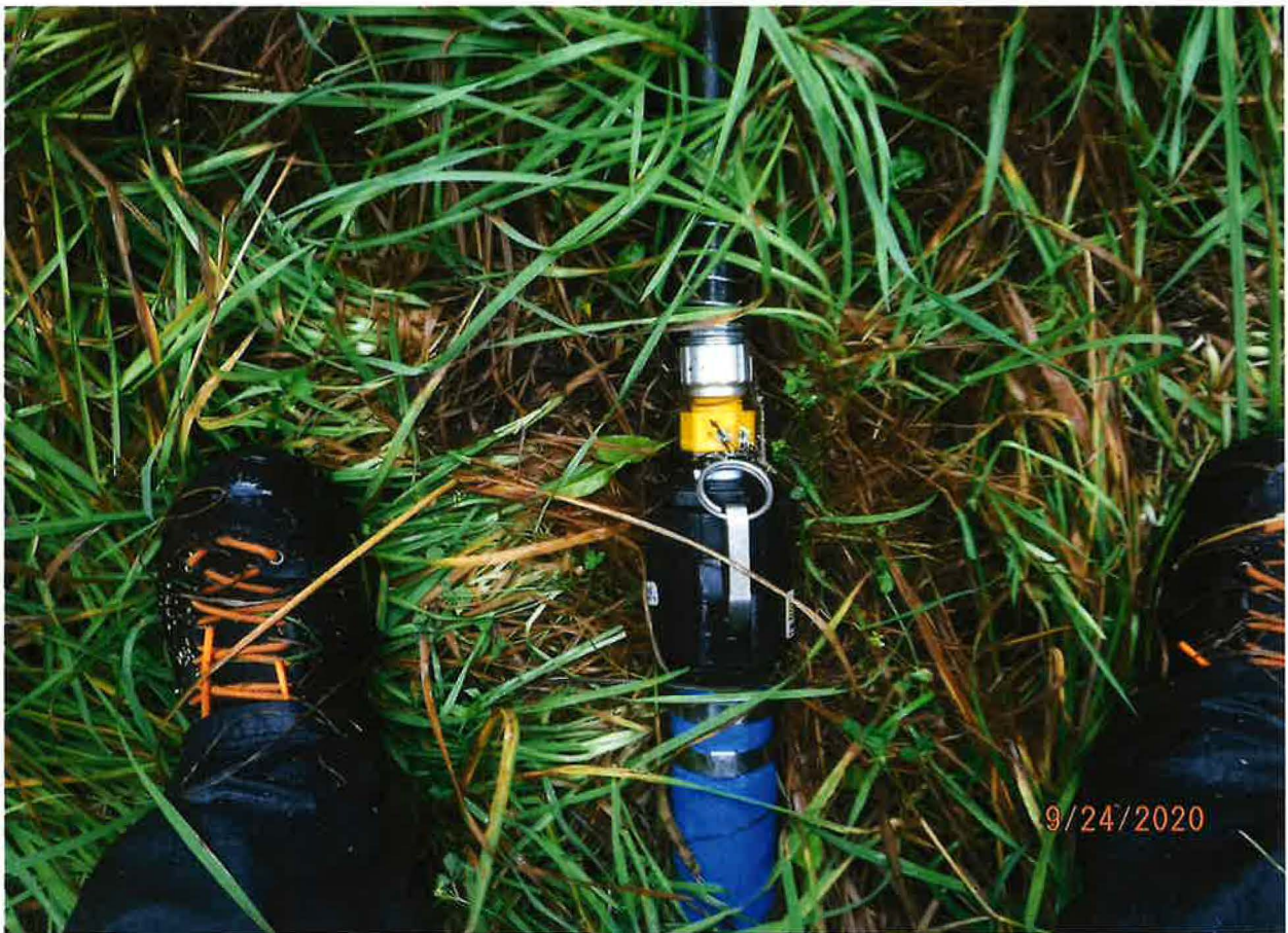
WATER CONVEYANCY SYSTEM – FIRE HOSE REDUCED DOWN TO GARDEN HOSE ATTACHMENT
