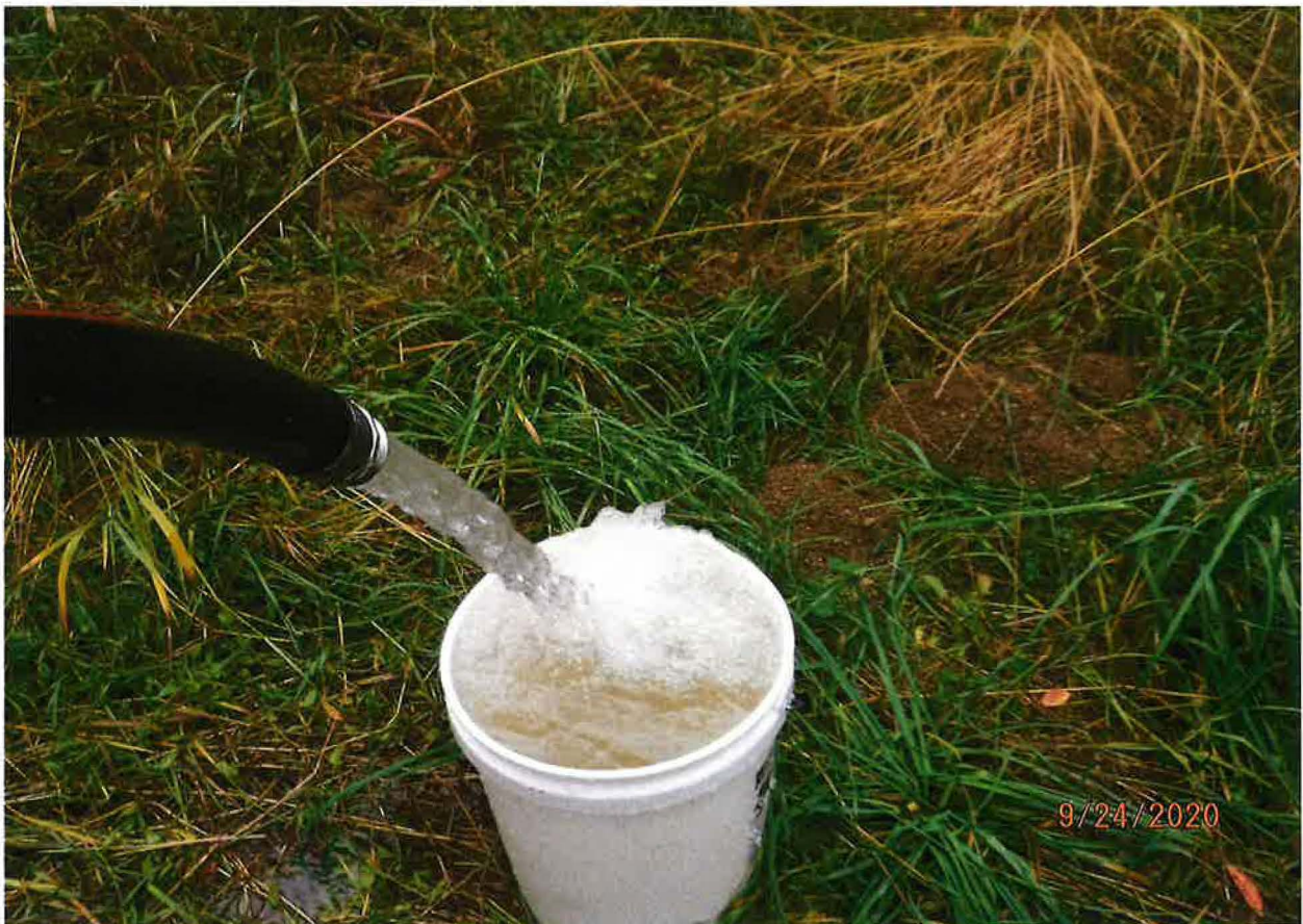
5 GAL BUCKET TESTS 3EA COMPLETED FOR FLOW MEASUREMENT
