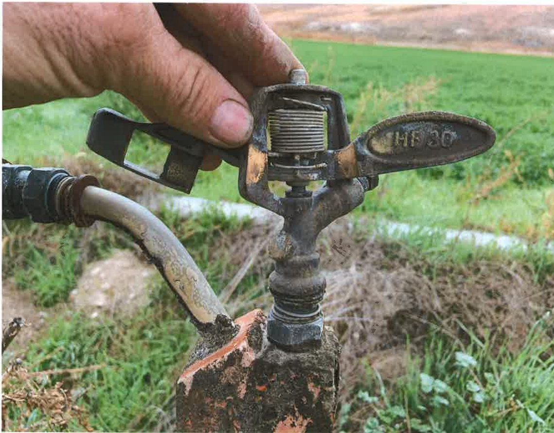
Fig. 9 – Sprinklers on hand-lines are Aquaburst HF 30 with 1/8" nozzle.
