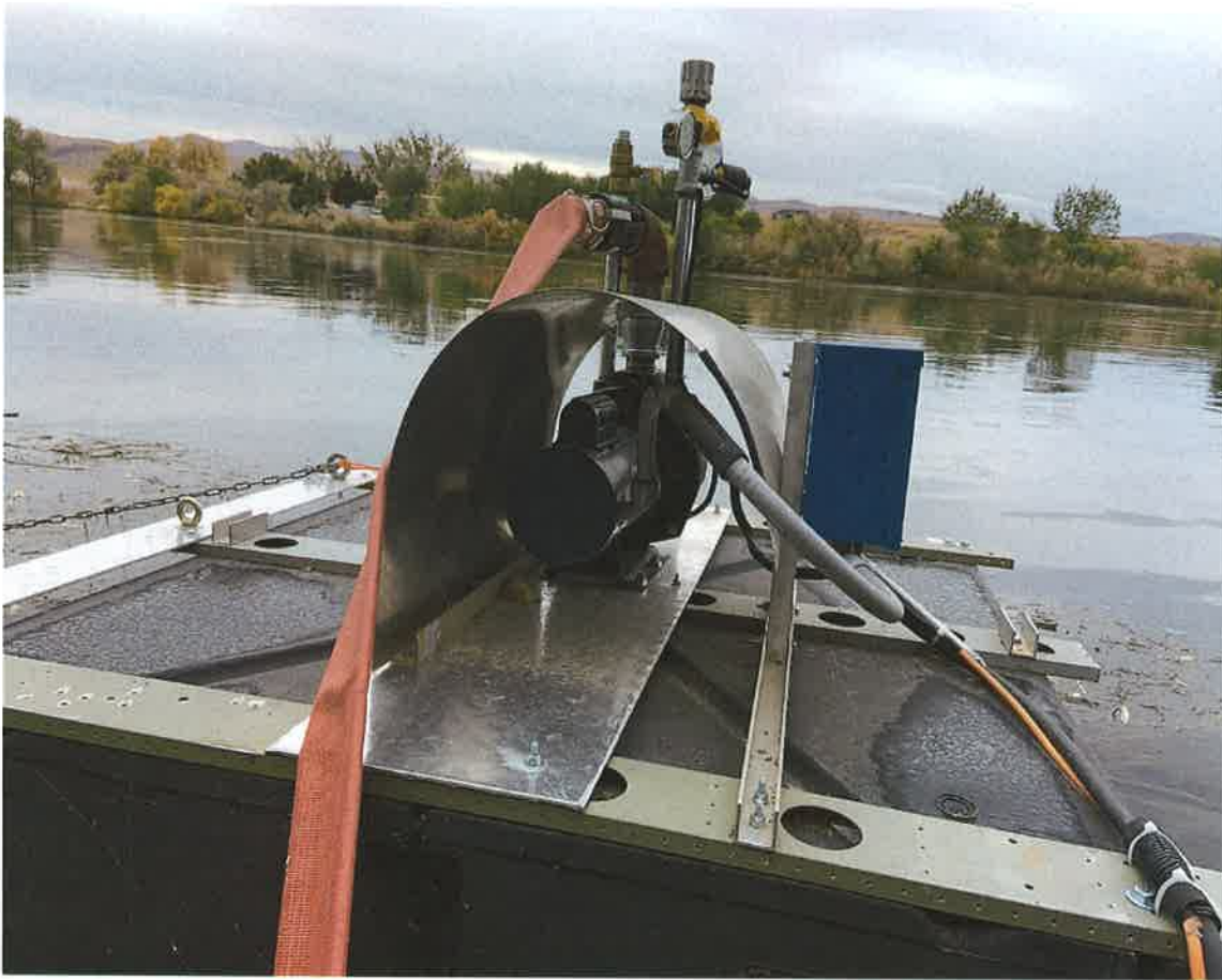
Fig. 3 – Alternate view of floating pump with 2" line coming from it.
