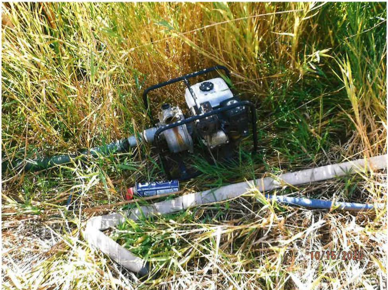
IRRIGATION FROM STORAGE SYSTEM – SCREENED HOSE AND WATER TRANSFER PUMP
