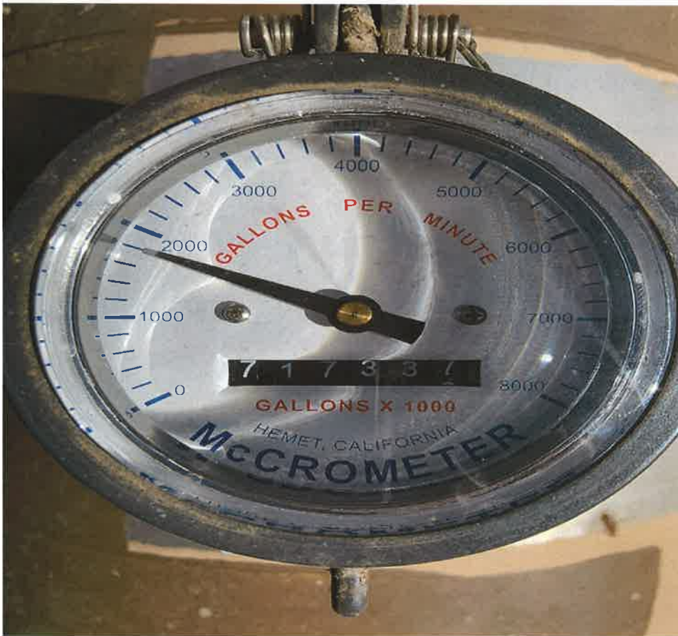
Fig. 9 – McCrometer measuring device for the right pump read an average of 2,000 gpm during the field exam.
