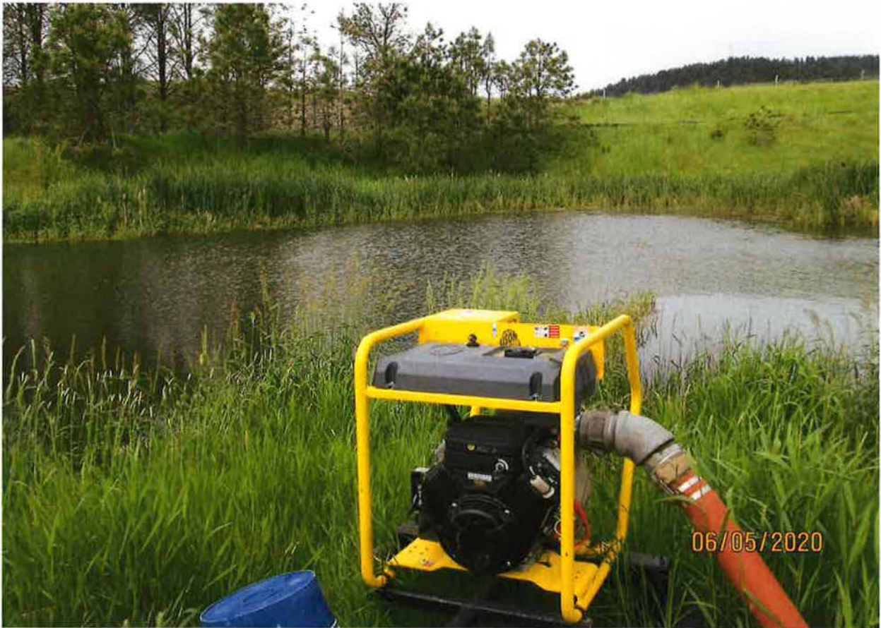
INDUSTRIAL FROM STORAGE PORTABLE WATER TRANSFER PUMP (16HP) WITH HOSE TO FILL WATER TRUCKS
