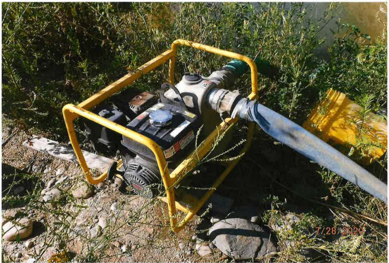
POD – HONDA GX 240 7 HP WATER TRANSFER PUMP
