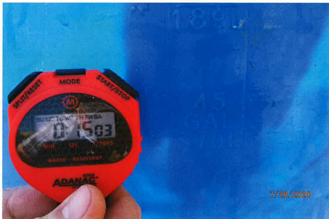
FLOW MEASUREMENT 45 GAL IN 15.03 SECONDS
