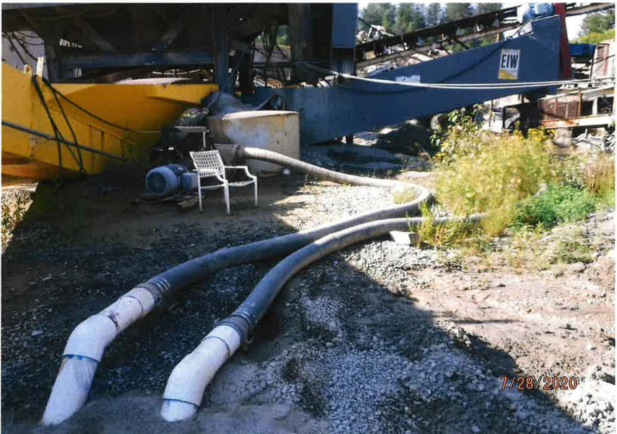
RECIRCULATION FEED PIPES FROM STORAGE POU TO INDUSTRIAL FROM STORAGE POU
