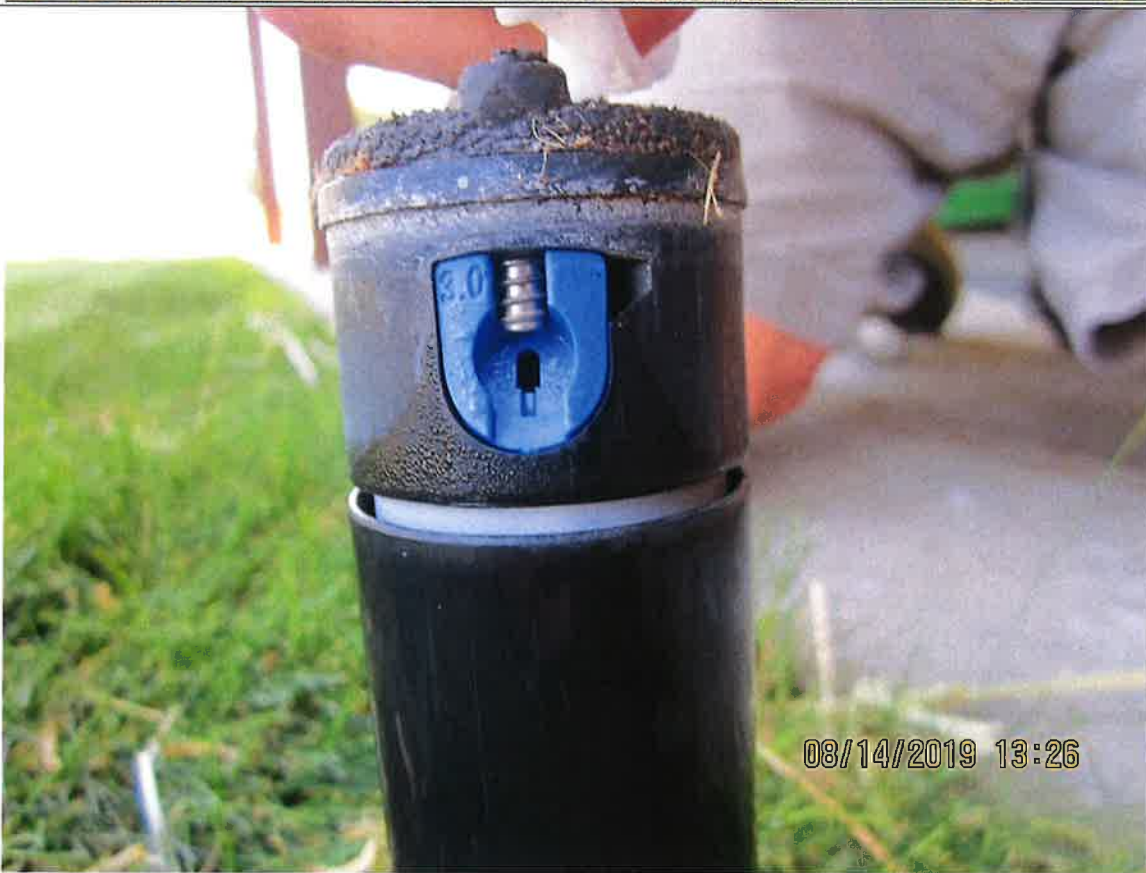
Figure 10. Pasture rotors were PGP Ultra Hunters with blue 3.0 gpm nozzles.
