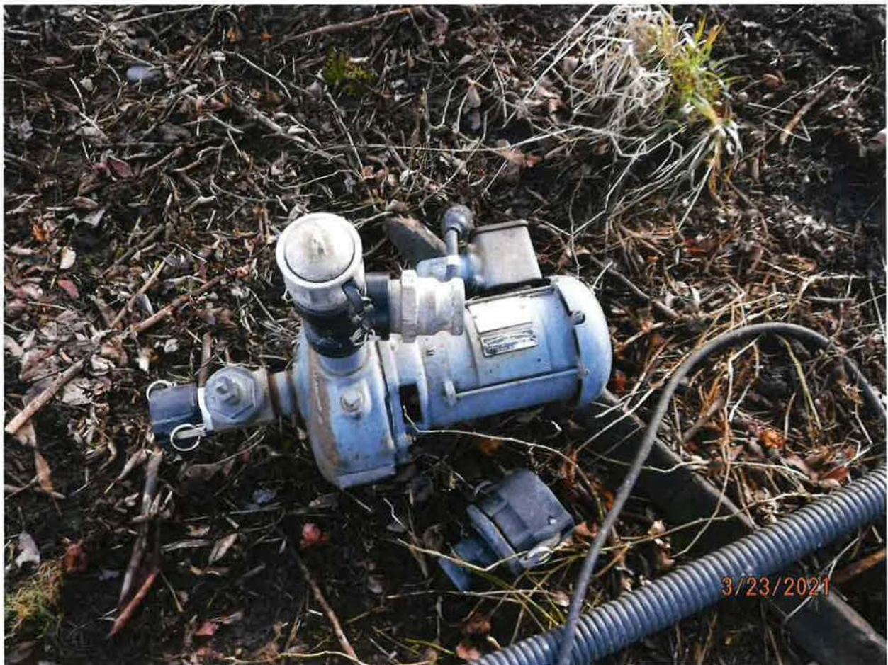
IRRIGATION FROM STORAGE – 30 FOOT FLOATING INTAKE PIPE TO PUMP
