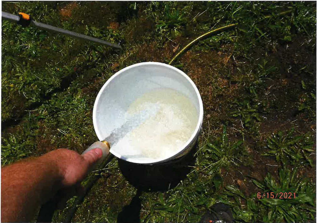
5 GAL BUCKET TEST FLOW MESUREMENT COMPLETED
