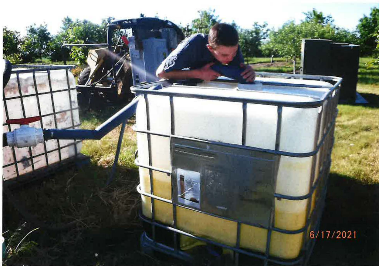
MULTIPLE FLOW MEASUREMENTS COMPLETED USING 275 GALLON TANKS LOCATED AT WELL
