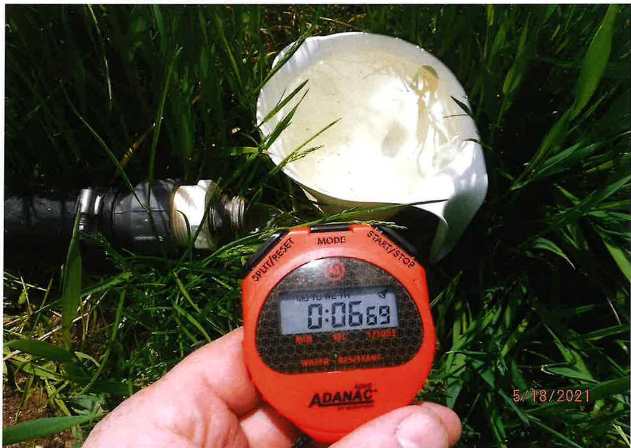
FLOW MEASUREMENT = 4 CUPS IN 6.69 SECONDS FROM END OF OVERFLOW DISCHARGE PIPE
