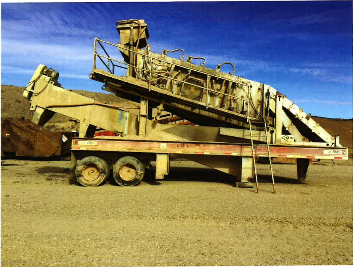
Gravel washing plant
