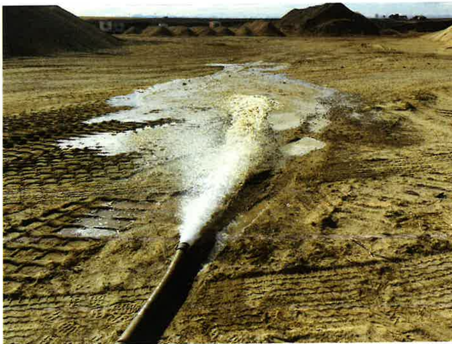
Fire hose discharge used for flow measurement
