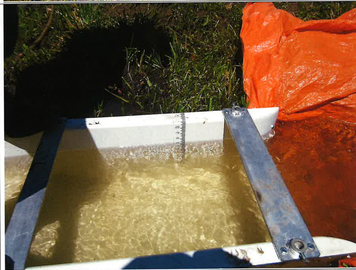
Figure 4. Initial broad-crested weir flume measurement with gage reading 15 cm or 1.49 cfs.
