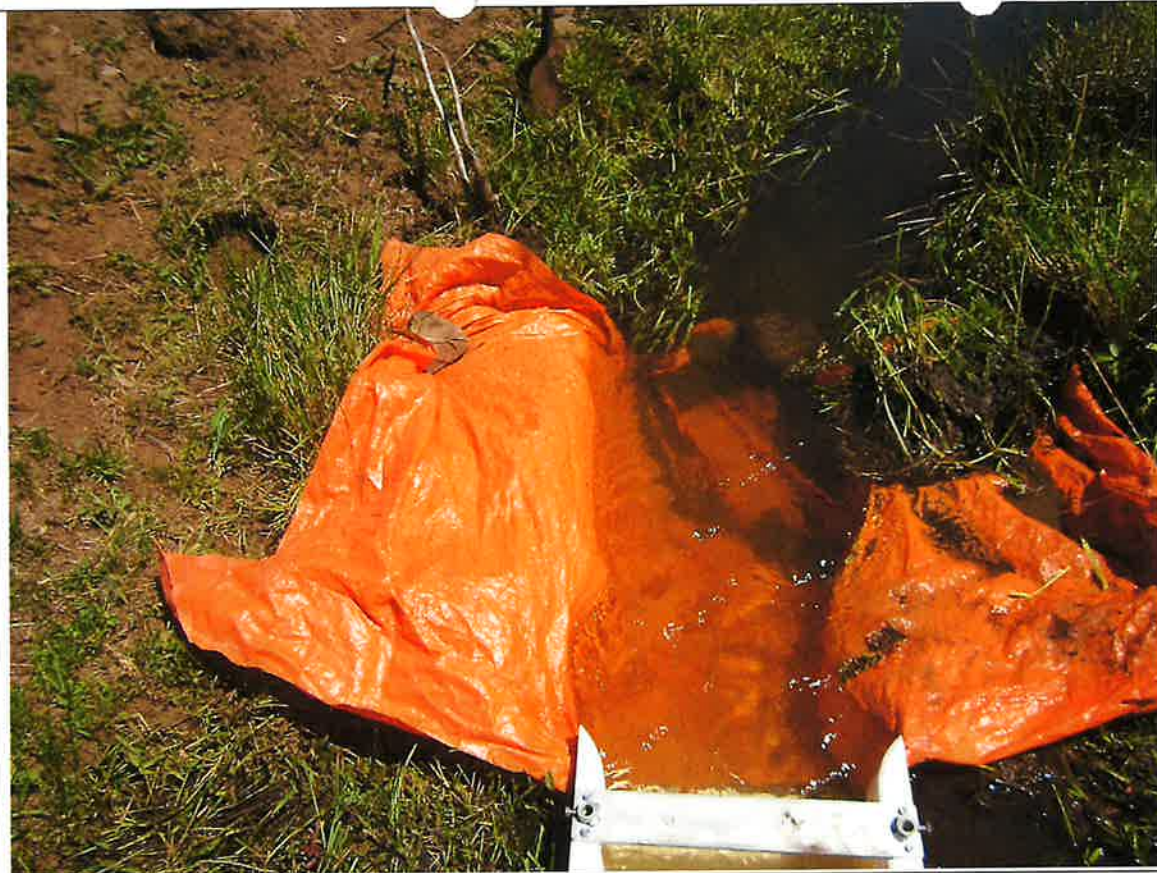
Figure 3. Upstream conditions for broad-crested weir flume measurement in north side ditch.
