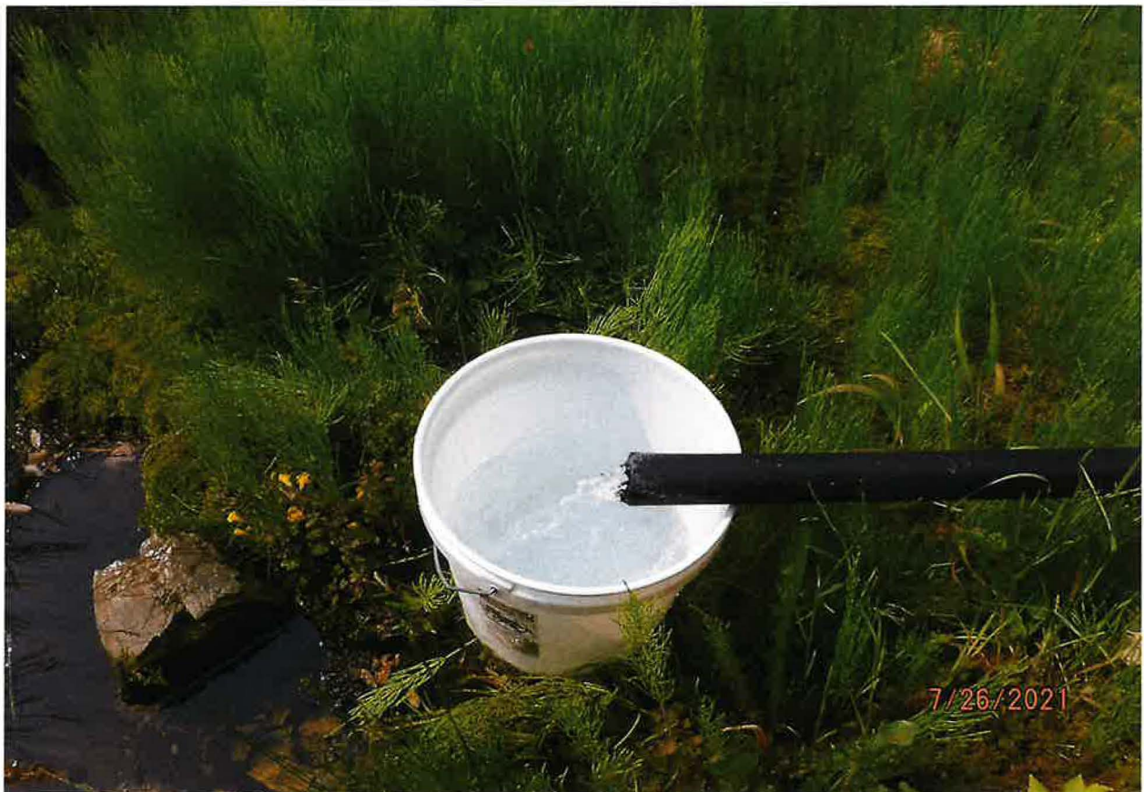
5 GALLON BUCKET FLOW MEASUREMENT
