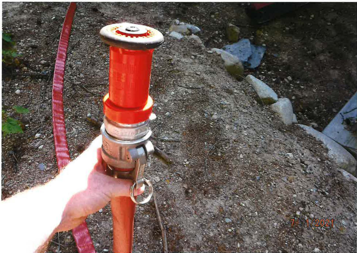
EXAMPLE FIRE SUPPRESSION SPRAY NOZZLE
