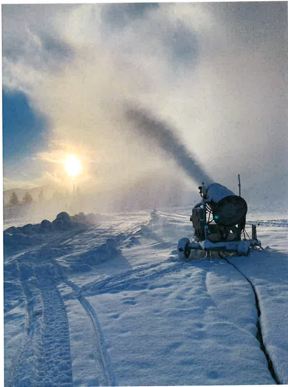
Photo 10: Snowmaking fan gun blowing run at Rotarun Ski Club Inc.'s facility in November 2020.
