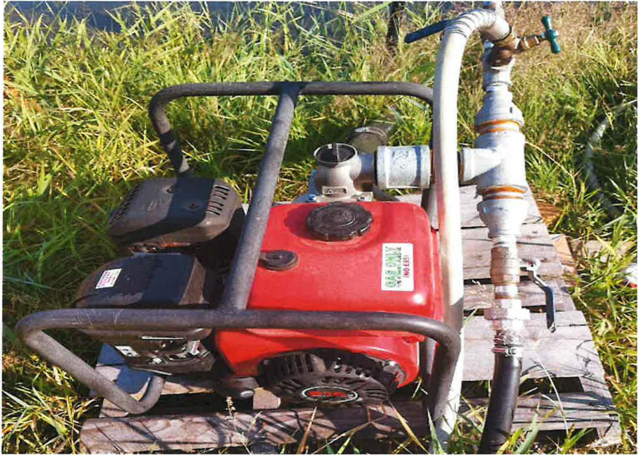
GENERATOR WATER TRANSFER PUMP DIVERTS WATER FOR IRRIGATION SYSTEM
