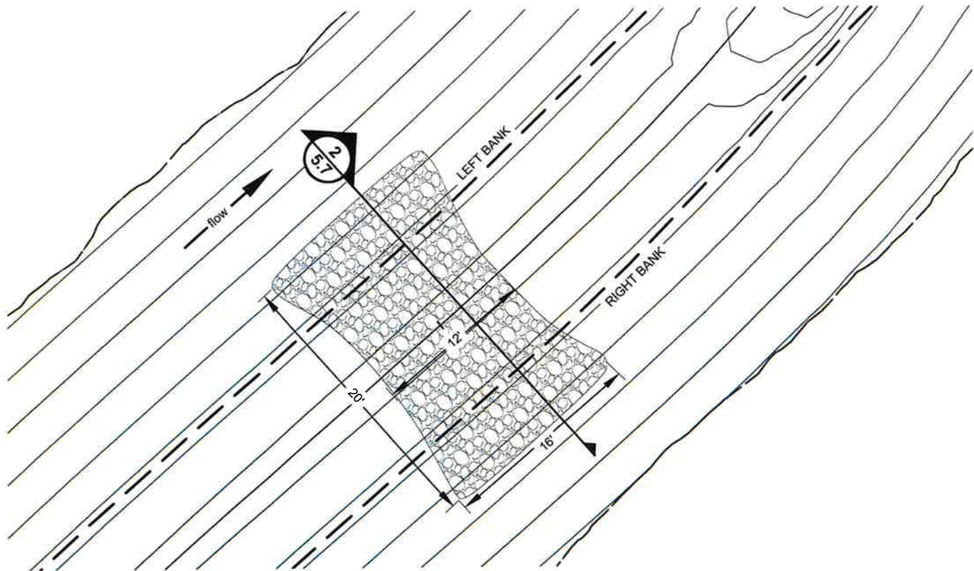
1 LOW WATER CROSSING PLAN VIEW 1" = 10'
