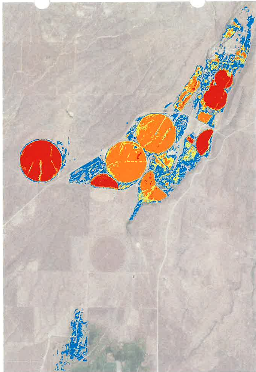
Figure 1 The raster image above shows NDVI values ranging from 0.6 (blue) to 0.88 (red)
