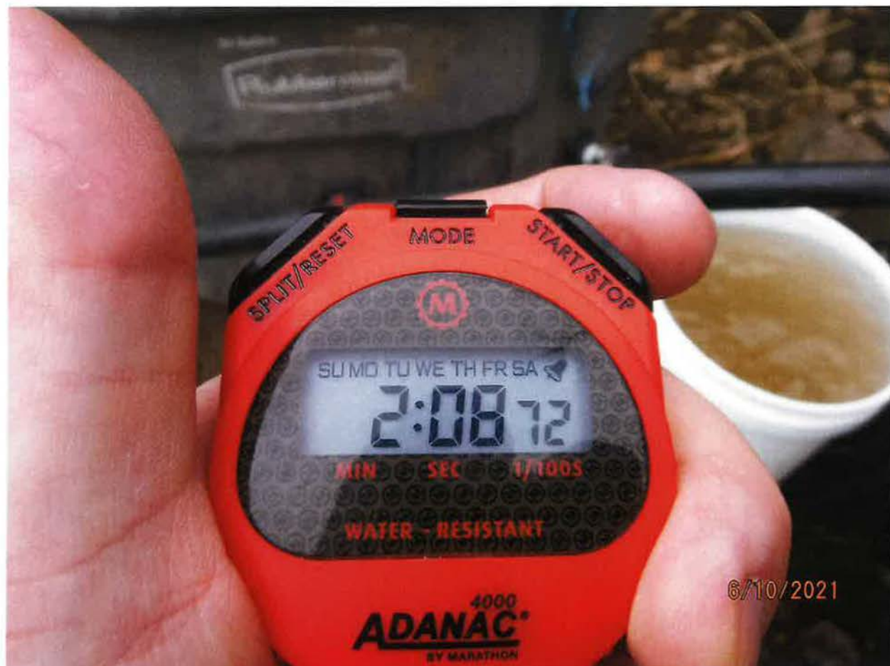
POD – 5 GAL BUCKET MEASUREMENT TAKEN FROM DIVERTING WORKS
