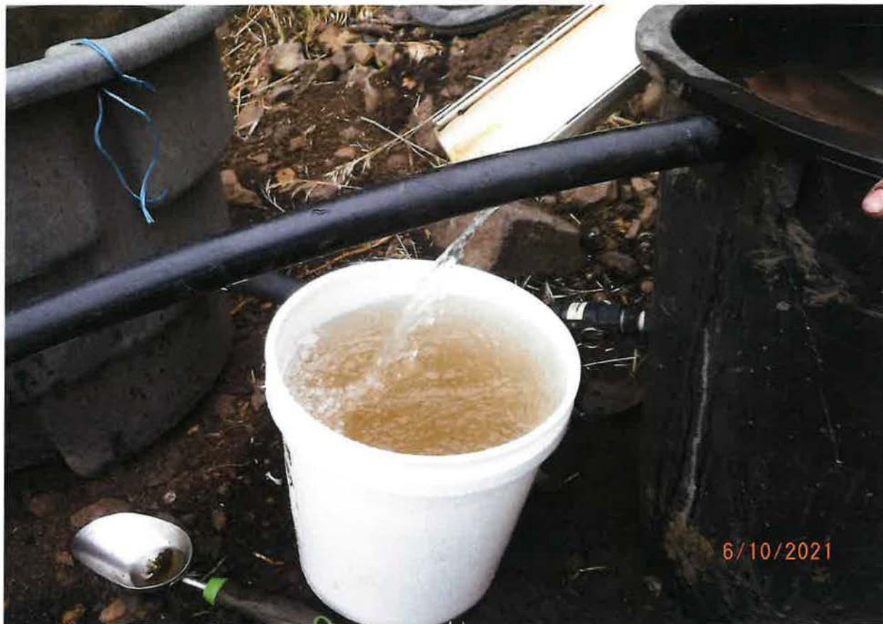
POD – 5 GAL BUCKET MEASUREMENT TAKEN FROM DIVERTING WORKS
