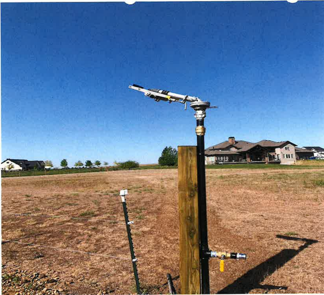
Fig. 7 – A Big Gun SR100 is installed in the pasture at the East end of the property. It was installed, but no beneficial use was developed from it during the development period.
