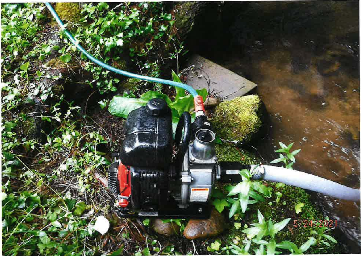
POD – 4 STROKE HONDA WATER TRANSFER PUMP, MODEL WX15T
