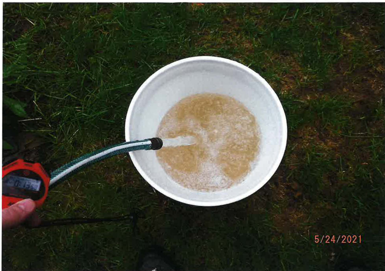
PERFORMING FLOW MEASUREMENT – 5 GAL BUCKET TEST FROM GARDEN HOSE AT POU
