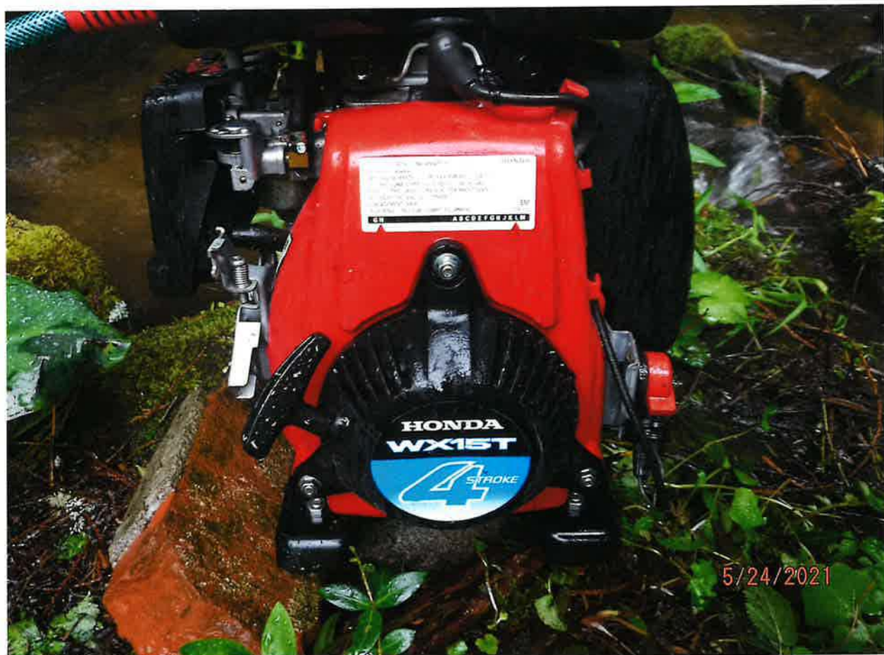
POD – 4 STROKE HONDA WATER TRANSFER PUMP, MODEL WX15T
