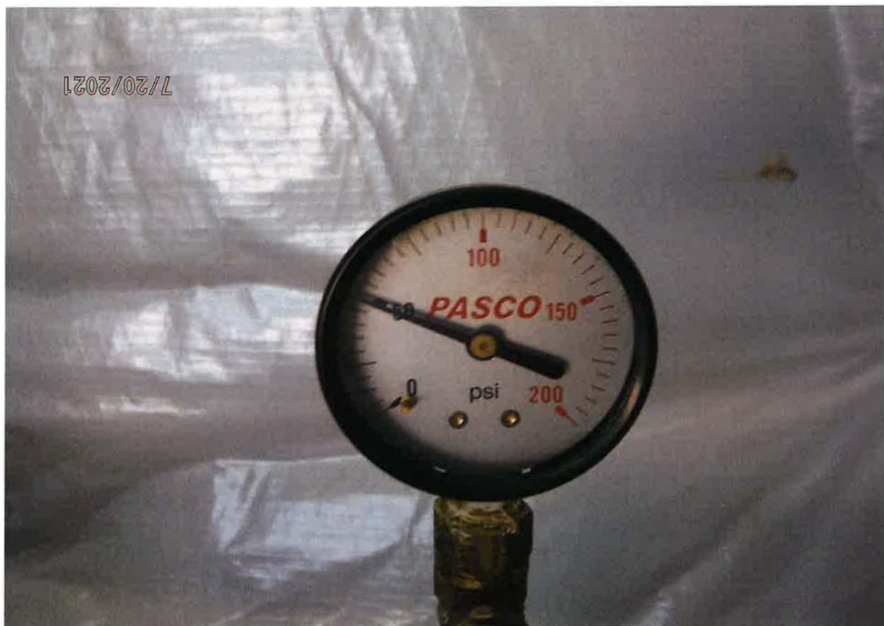
50 PSI SYSTEM OPERATING PRESSURE
