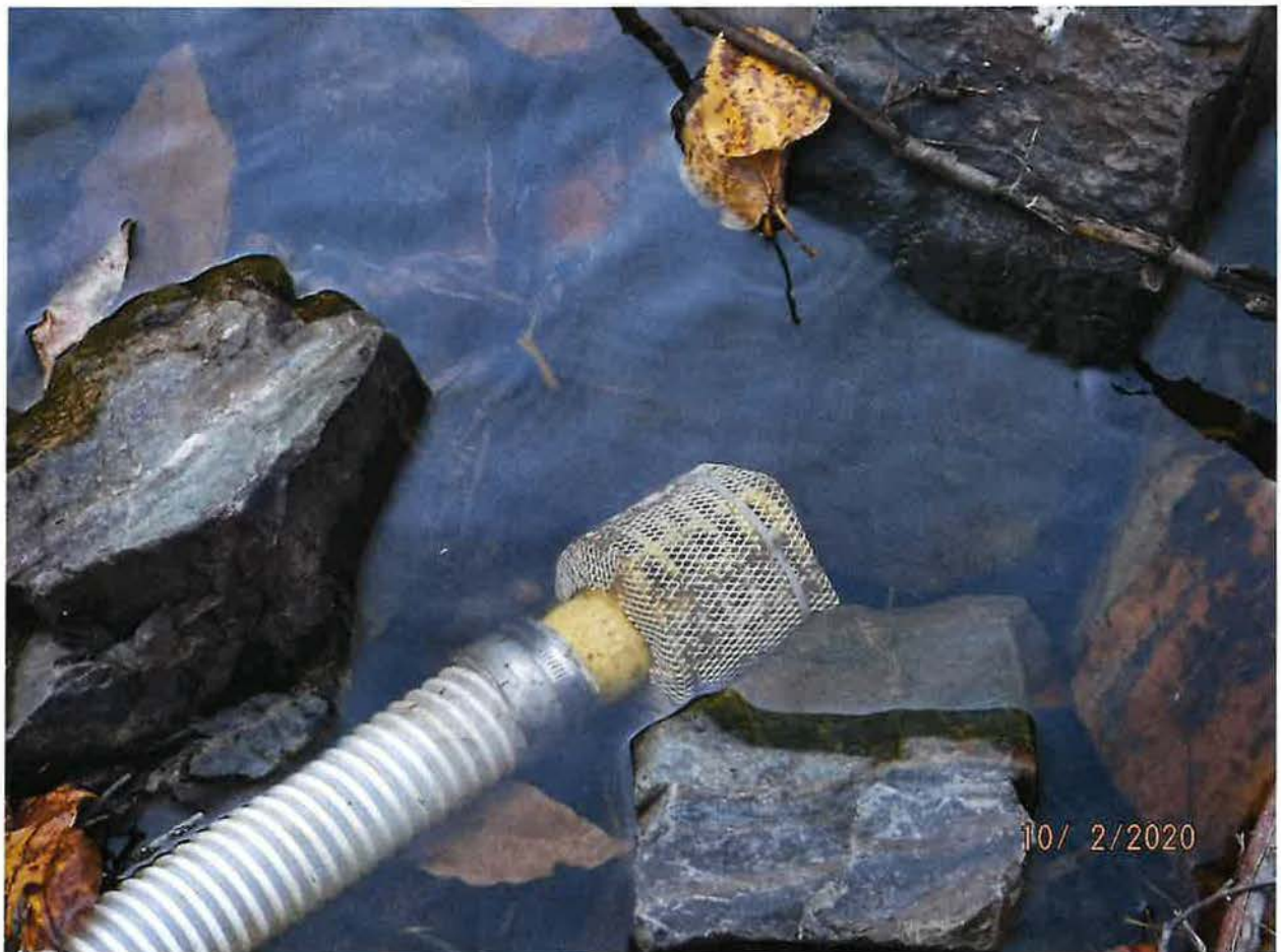
AT POD – SCREENED INTAKE SUCTION PIPE IN RIVER
