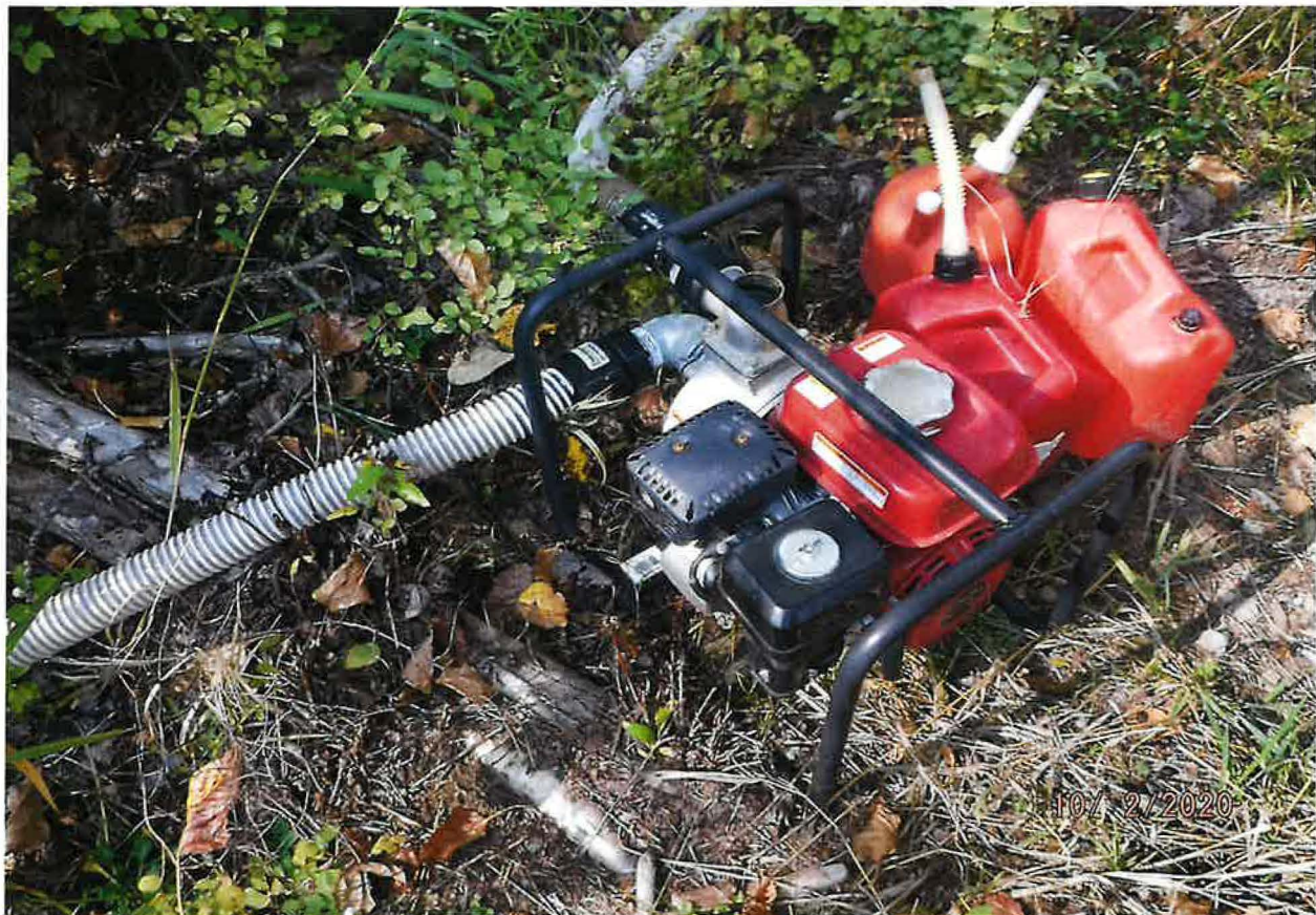
POD – HONDA WB20XT WITH GX120 MOTOR WATER TRANSFER PUMP 2" PORT
