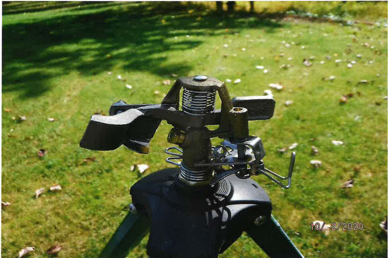
ORBIT BRASS IMPACT SPRINKLER 6EA OPERATES AT ONE TIME, ALTERNATES IRRIGATION SCHEDULE
