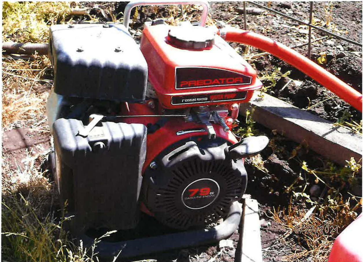
SMALL WATER TRANSFER PUMP FROM 24 HR IMPOUNDMENT FOR IRRIGATION USE
