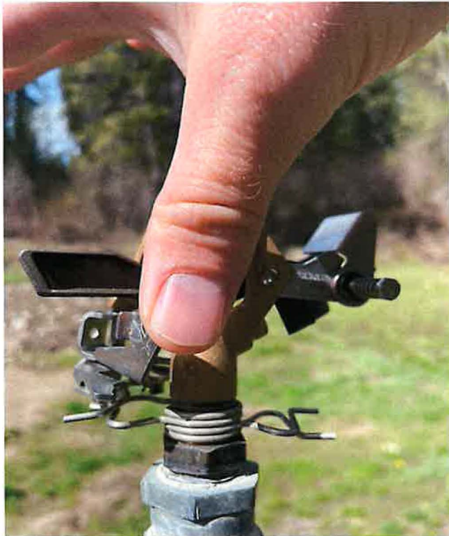
Fig. 5 – Rainbird B impact sprinklers with PJ nozzle on hand-lines.
