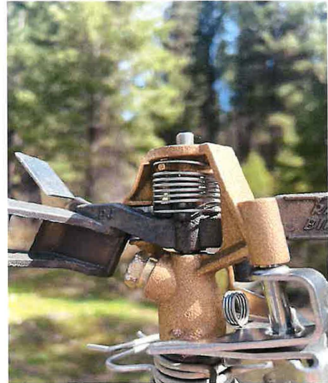
Fig. 6 – Rainbird B impact sprinklers with PJ nozzle on hand-lines.
