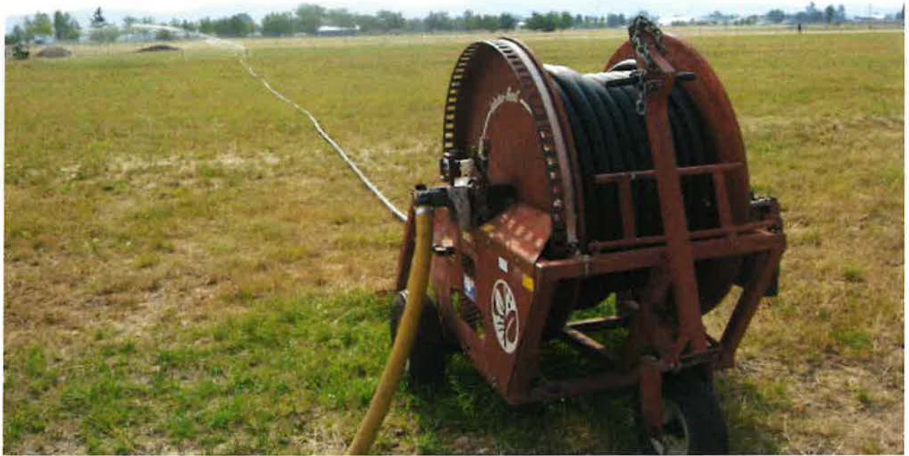
IRRIGATION POU – BIG WHEEL SPRINKLER FROM MAIN TRUNK HAND LINE AT HAY FIELD
