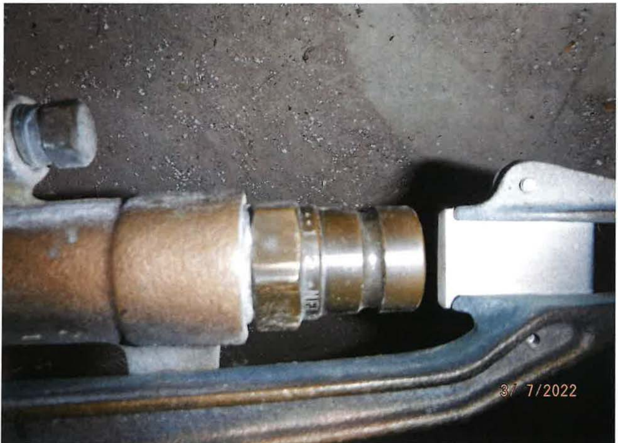
WATER REEL WITH 1/2 INCH IRRIGATION NOZZLE INSTALLED
