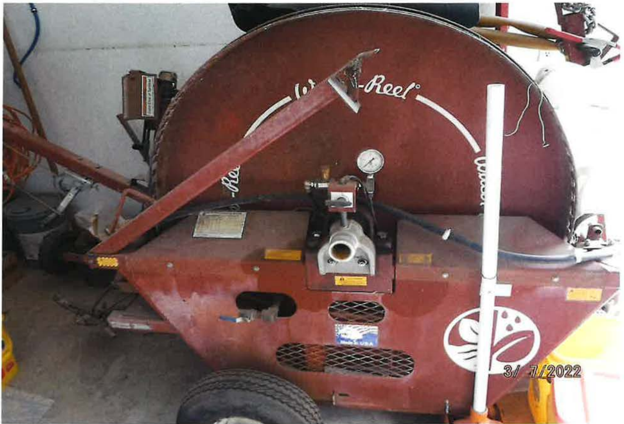
WATER REEL WITH 1/2 INCH IRRIGATION NOZZLE INSTALLED
