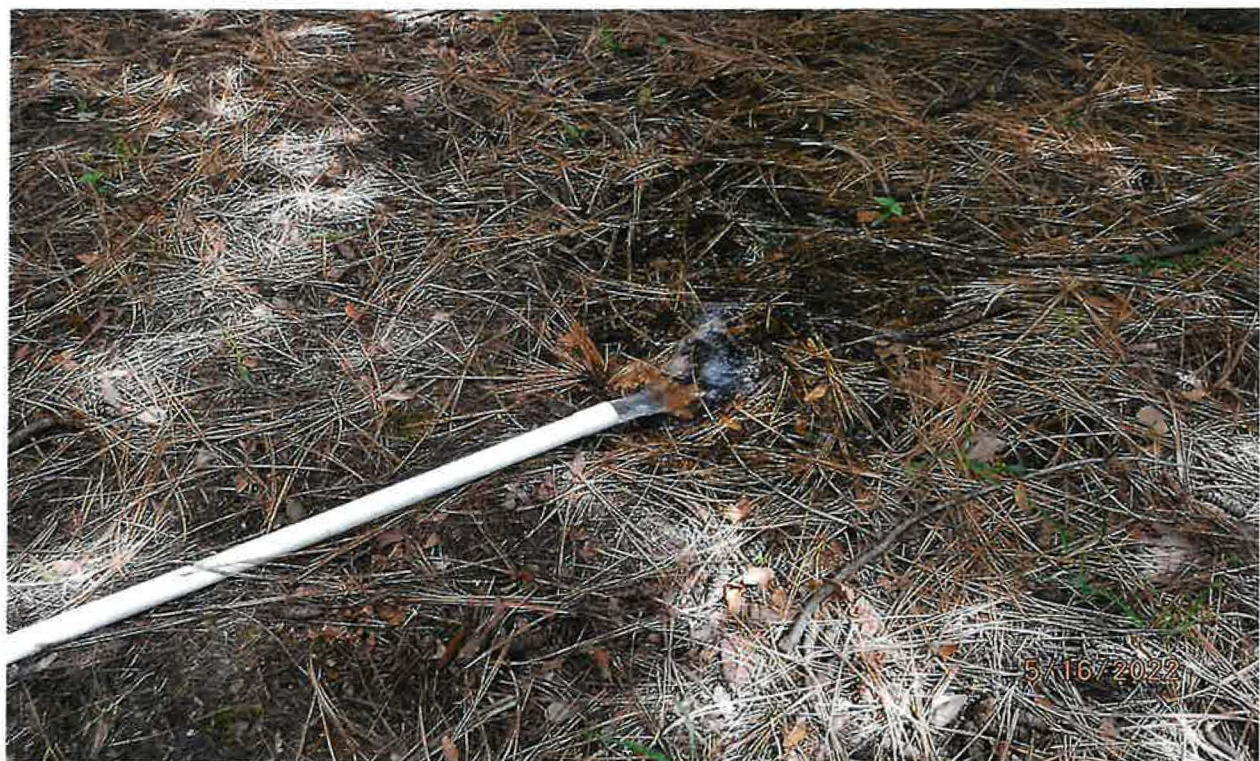
INDIVIDUAL PARCEL SPRINKLER BLOW OUT PIPE
