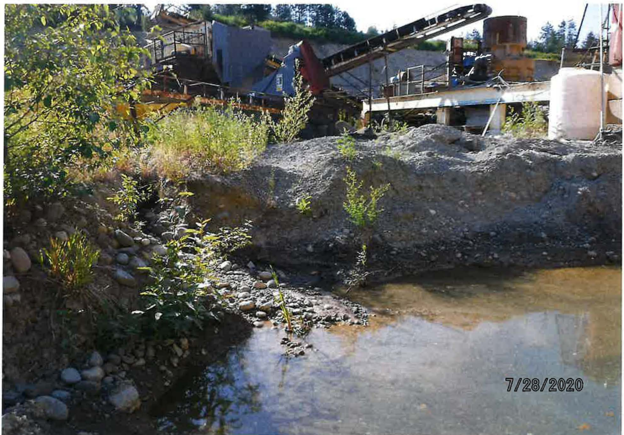
OVERFLOW FROM AGGREGATE WASHING RECYCLED BACK TO OPEN PIT WELL FOR USE
