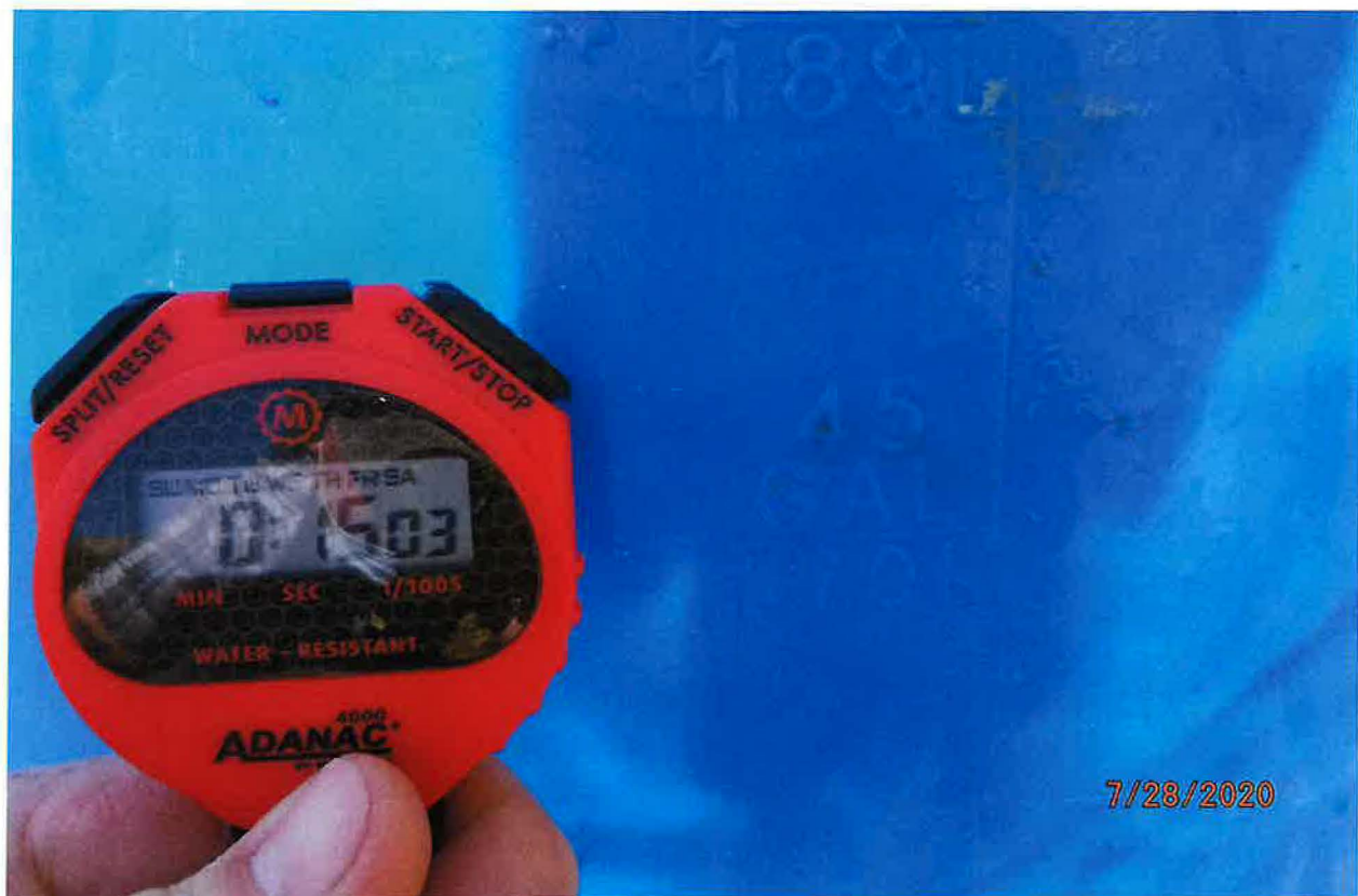
FLOW MEASUREMENT 45 GAL IN 15.03 SECONDS
