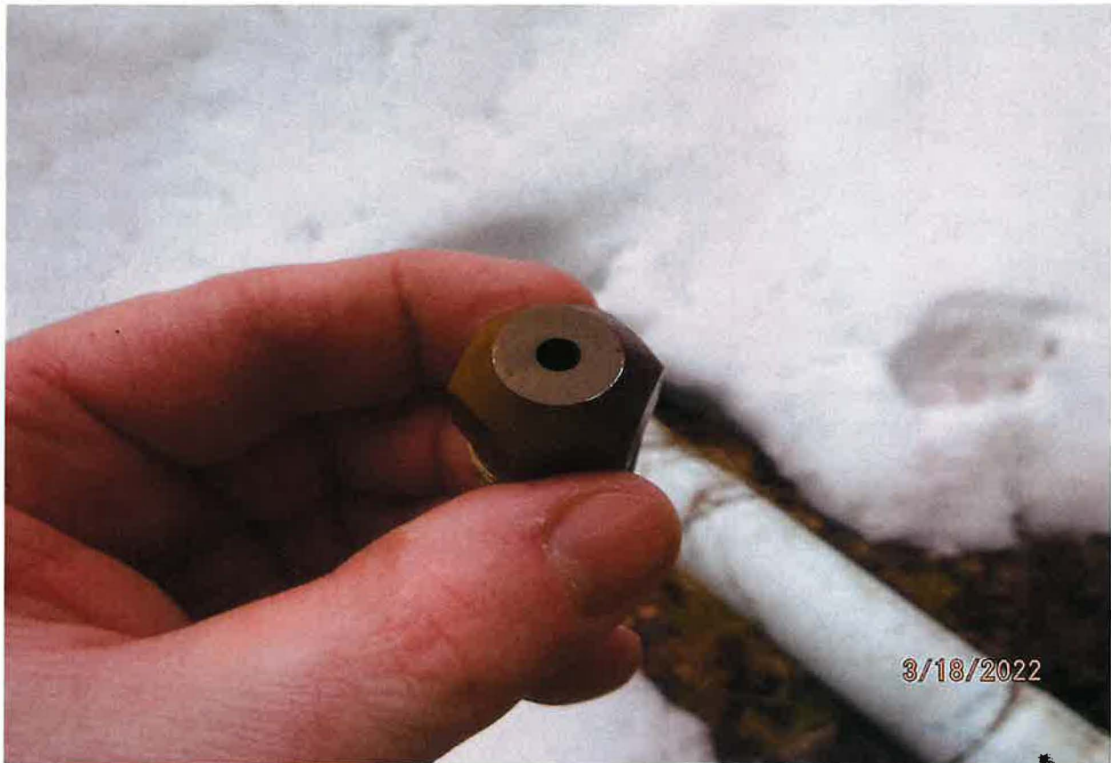
1ea 3/16" NOZZLE – MISMATCHED IN SYSTEM ASSUMED TO BE 1/4"; MICROMETER MEASUREMENT VALIDATED.
