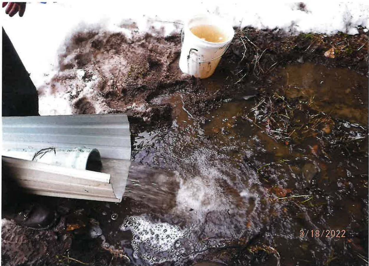
OVERFLOW DISCHARGE AREA HAND DUG TO ALLOW MULTIPLE 5-GAL BUCKET MEASUREMENTS
