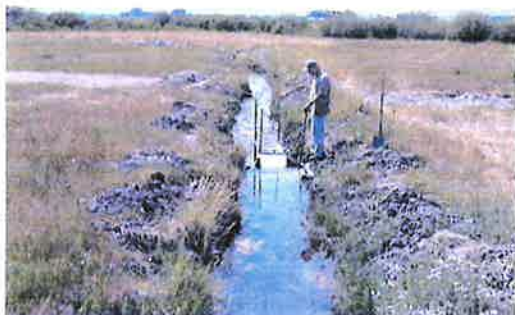
Portable flume in ditch flowing west.
