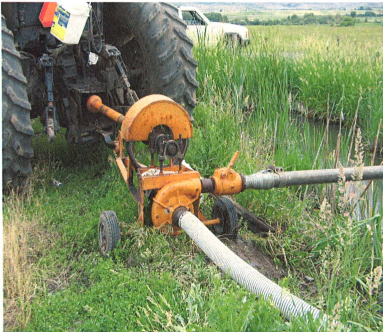
View of PTO pump (on neighbor's property)
