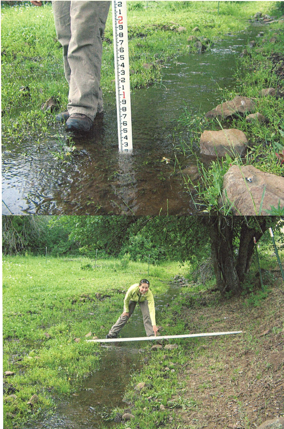
Cursory measurement of ditch from A0017648. Ditch was 2.5 inches deep by 4 feet wide. Field examiner in lower picture is pointing to 4-foot mark. Mr. Hoffman states the ditch is normally this wide, but is usually 6-8 inches deeper during active irrigation.
