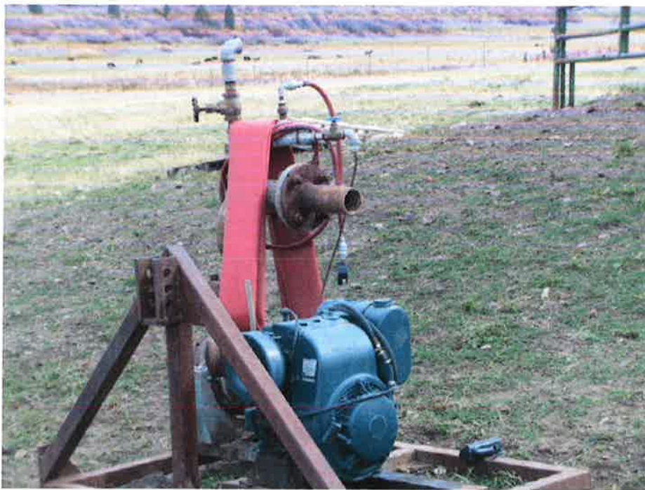
Photo 1. Looking south at portable pump. Kohler engine, 14 hp. Serial number 10032490, model number K321T.
