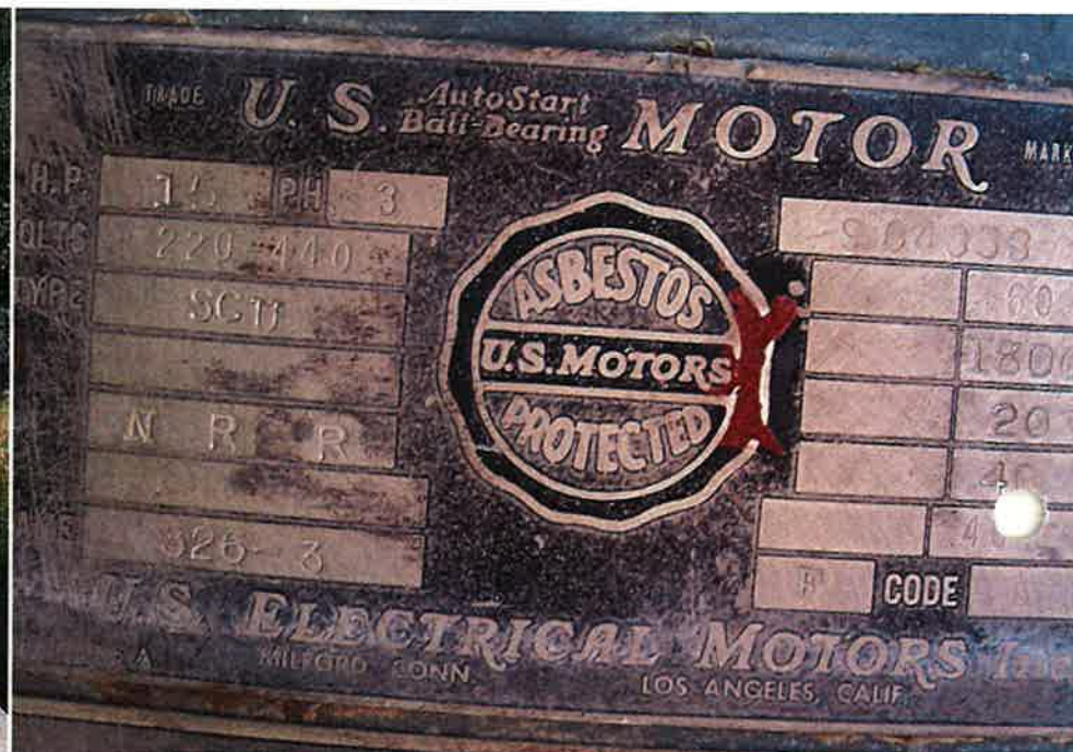
US Motor 15 Hp turbine
