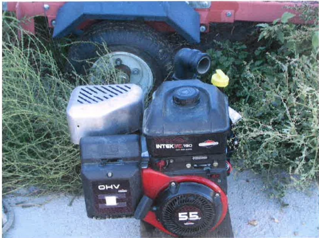
Photo 3. Briggs and Stratton 5.5 hp portable pump with 4-inch hand lines. Donald Hall also uses this system.
