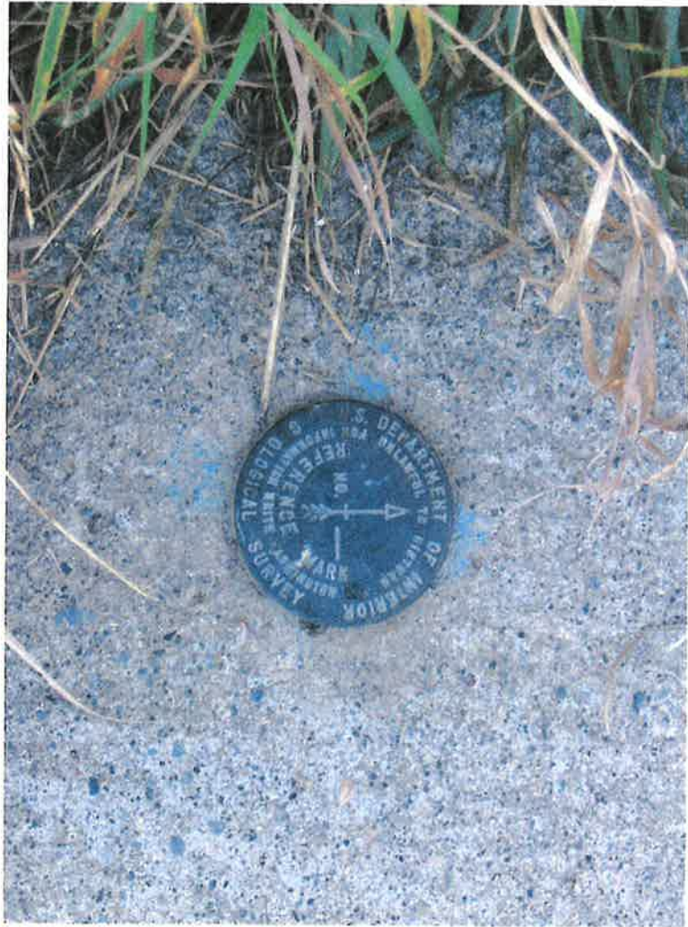
A22-12528 & A22-634; Survey marker on pump pad
